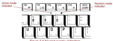
Figure 2-9 Keypad overlay indicators
